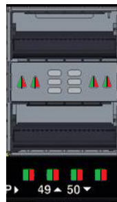
Figure 11. QSFP28 Port LEDs
