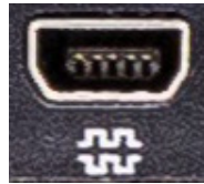
Figure 4. RS-232 Mini-USB serial port
