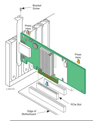
**NOTE:** The shape, size, and locations of components on your controller and its bracket might vary from this illustration. The controller requires an x8 PCIe slot. Some PCIe slots support only PCIe graphics cards; a controller installed in one of these slots will not function. Refer to the guide for your motherboard for information about the PCIe slot.
