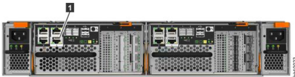
Figure 29. Lenovo Storage V7000 technician port
