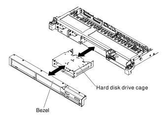
Figure 76. Hard disk drive cage installation
