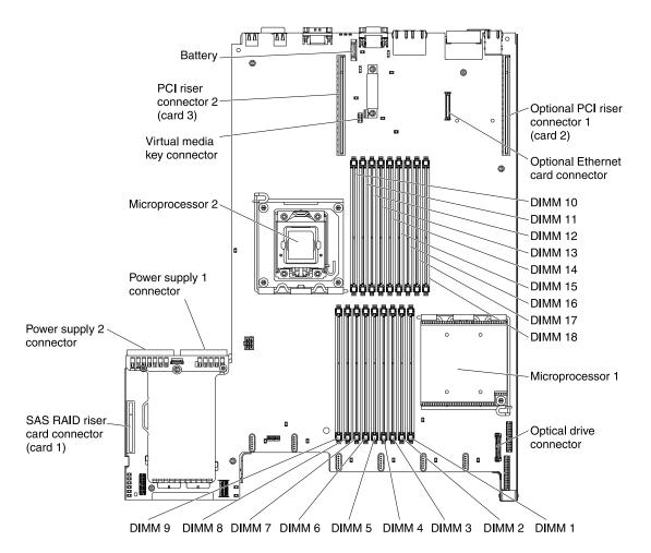
Figure 19. System-board optional device connectors
