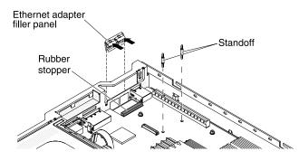
Figure 59. Filler panel removal
