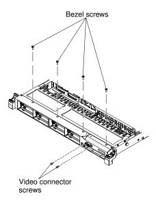
Figure 75. Screws removal
