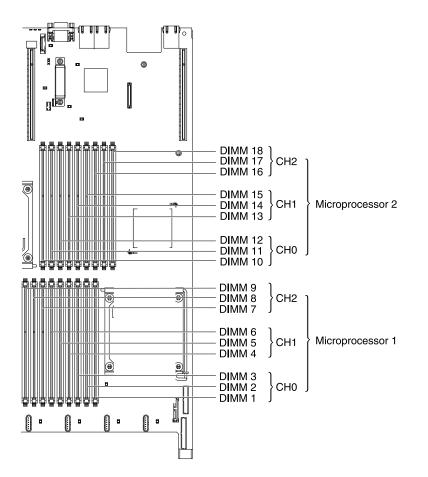
Figure 29. DIMM connectors location
