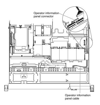
Figure 22. Operator information panel cable connection
