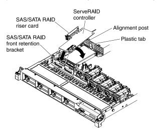
Figure 45. ServeRAID controller installation
