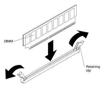
Figure 32. DIMM installation
