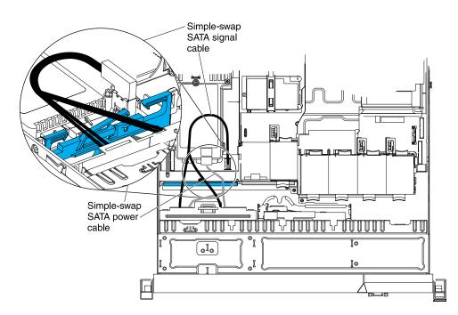
Figure 24. Simple-swap backplate assembly cable connection
