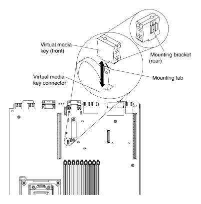
Figure 57. Virtual media key installation
