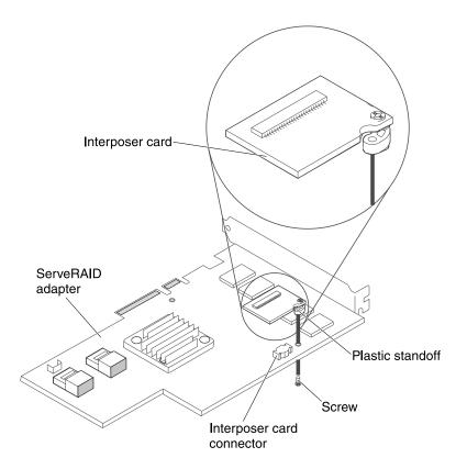
Figure 65. Interposer card installation
