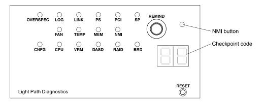
Figure 8. Light path diagnostics panel exposure
