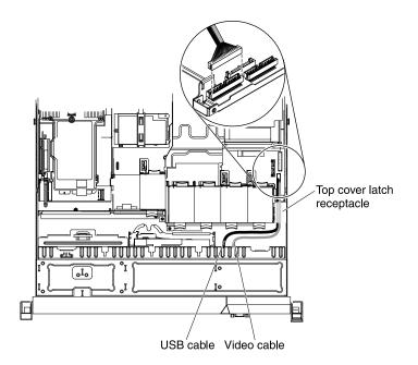
Figure 23. USB/video cable connection
