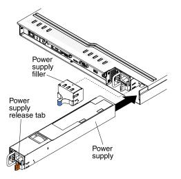
Figure 54. Power supply installation
