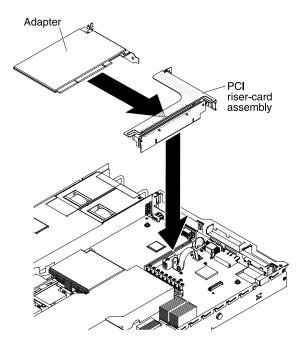
Figure 42. Adapter installation
