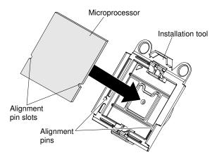
Figure 79. Microprocessor alignment
