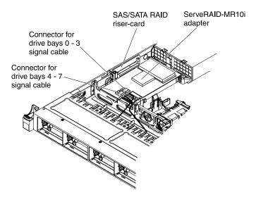
Figure 49. ServeRAID-M10i adapter cable connection
