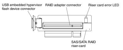
Figure 43. RAID adapter connector
