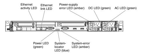
Figure 10. Rear view LEDs
