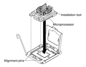
Figure 81. Microprocessor installation
