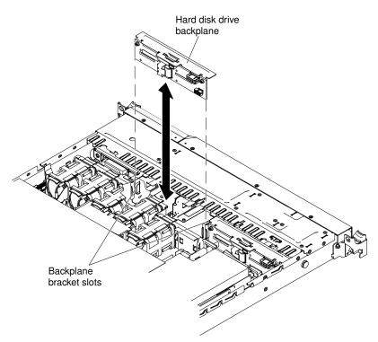
Figure 77. Hard disk drive backplane installation
