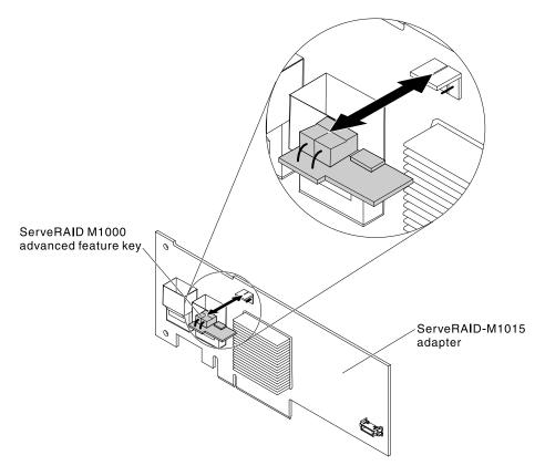
Figure 50. ServeRAID M1000 advanced feature key installation
