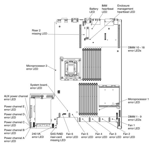
Figure 18. System-board LEDs
