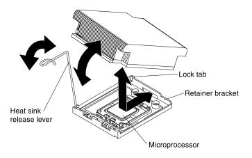
Figure 84. Heat sink installation
