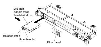
Figure 35. Simple-swap hard disk drive installation
