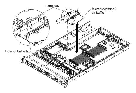
Figure 28. Microprocessor 2 air baffle removal
