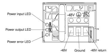
Figure 11. DC power supply LEDs
