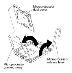
Figure 78. Dust cover removal
