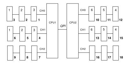
Figure 30. Memory channel interface layout
