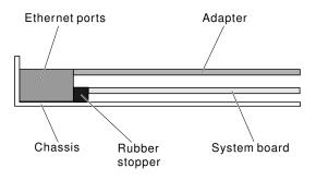
Figure 62. Adapter installation
