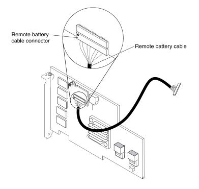
Figure 66. Cable connection
