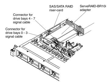
Figure 47. ServeRAID-BR10i adapter cable connection
