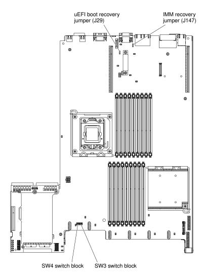
Figure 17. System-board switches and jumpers
