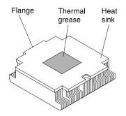
Figure 83. Thermal grease
