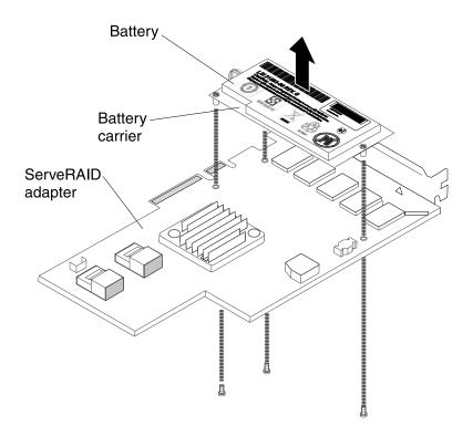
Figure 64. Battery removal
