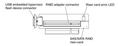
Figure 93. USB embedded hypervisor flash device connector
