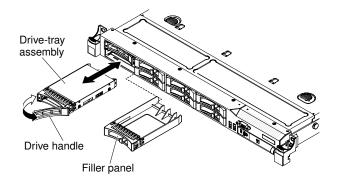
Figure 33. Hot-swap hard disk drive installation
