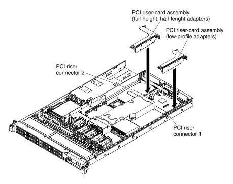
Figure 41. PCI riser-card assembly installation
