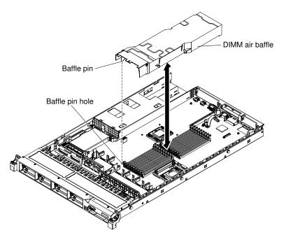
Figure 88. DIMM air baffle installation
