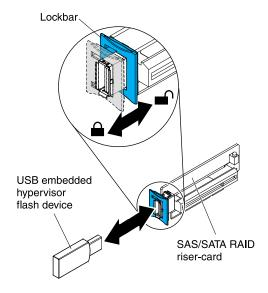
Figure 56. USB embedded hypervisor flash device installation
