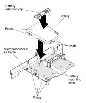
Figure 70. Battery installation
