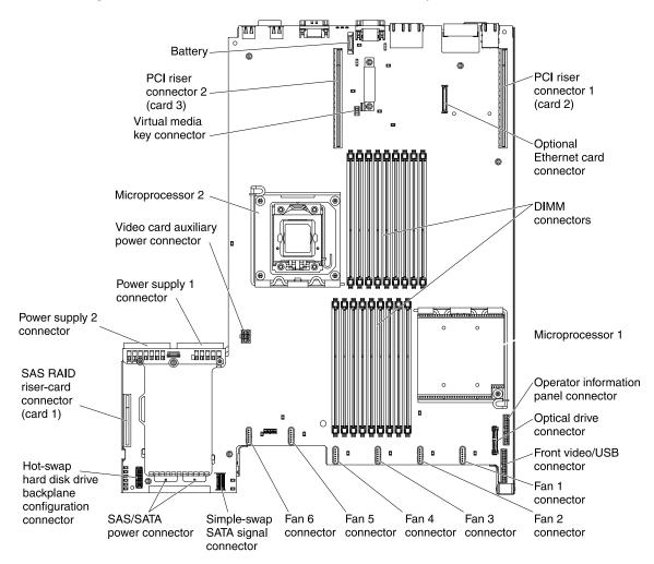
Figure 15. System-board internal connectors
