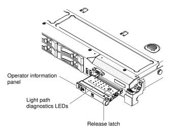
Figure 7. Light path diagnostics panel exposure
