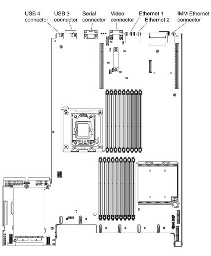
Figure 16. System-board external connectors
