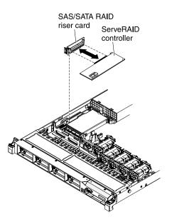
Figure 44. ServeRAID controller installation
