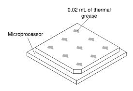
Figure 85. Thermal grease distribution
