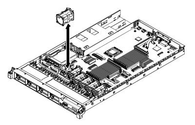
Figure 53. Fan installation
