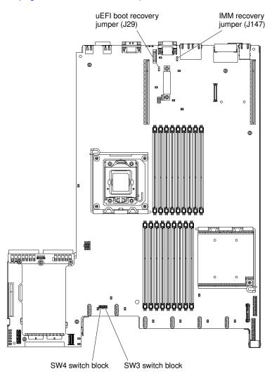
Figure 92. System-board switches and jumpers
