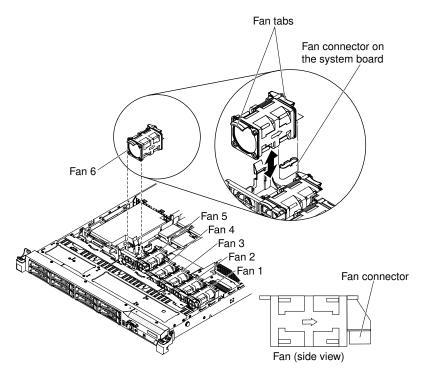
Figure 52. Fan installation
