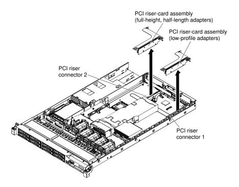
Figure 40. PCI riser-card assembly removal
