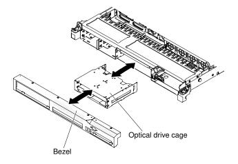
Figure 72. Optical drive cage installation
