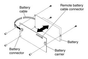
Figure 69. Cable connection
