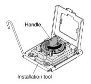
Figure 82. Installation tool handle adjustment
