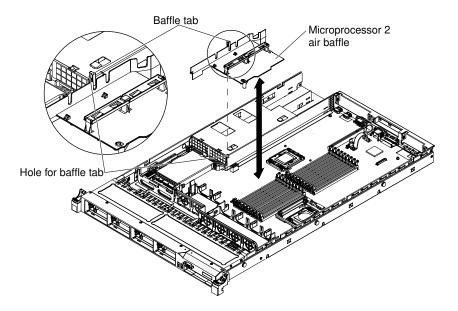
Figure 87. Microprocessor 2 air baffle installation
