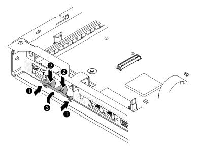
Figure 60. Metal clip installation
