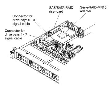
Figure 20. ServeRAID adapter cable connection
