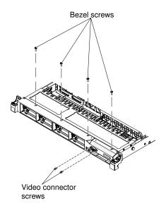
Figure 71. Screws removal
