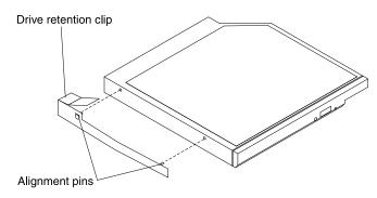
Figure 38. DVD drive retention clip installation
