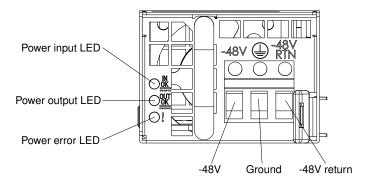
Figure 13. DC power-supply LEDs
