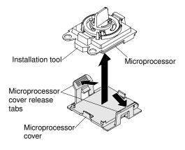
Figure 80. Microprocessor cover removal
