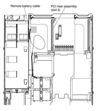
Figure 67. Cable connection
