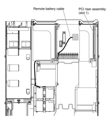
Figure 68. Cable connection
