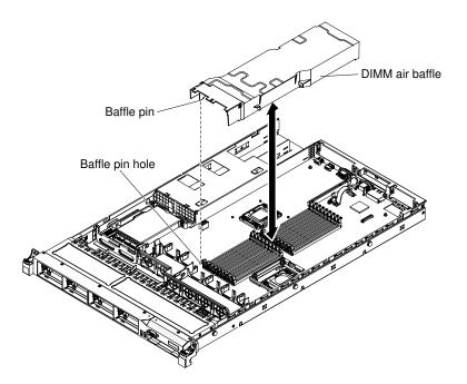
Figure 27. DIMM air baffle removal
